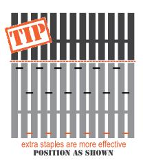
Before making your cut, secure each slat by driving a crown staple with a hammer or power gun to bridge the gaps.
