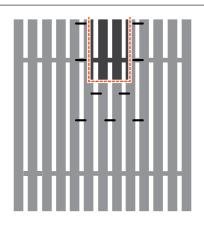
(Option B) If the cut you are making is on the edge of the tile, step 2 (Option A) can be ignored. Simply make your measurements on the back of the tile (in reverse) and proceed to step 3
