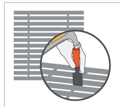
Note: If a tile falls in a horizontal relationship to the boundary and requires resizing, you may split the PVC tubing with a chisel of knife to allow for an accurate fitting.
