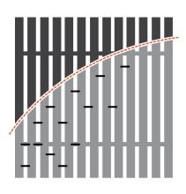
Before cutting, secure the back of the tile with crown staples and stagger them.
