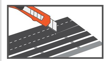
In order to compensate for uneven surfaces, levelling your product may be necessary. We highly recommend the use of roofing shingles for this purpose. Before proceeding with the installation, cut your sheets up into 1–1.5" wide strips accordingly.
