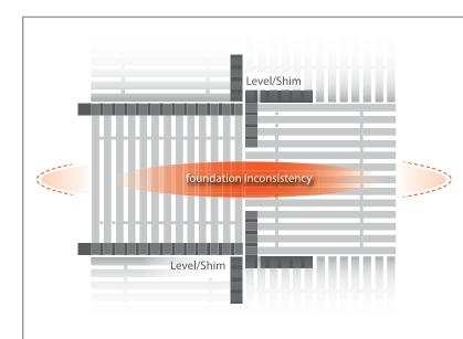
Use your levelling strips to compensate for uneven surfaces, bumps, obstructions. As if the tile were a teater-totter mounted on a fixed point (the bump) use these strips on either end if not both to stop the rocking motion. Furthermore, stacking the material will give you the ability conform to any irregularity the tile(s) are positioned on top of.
