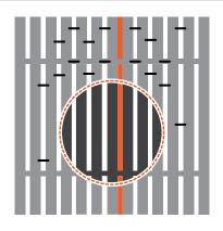
(Option A) If you'd like to wrap your tile around an obstruction such as a post, split the tile in half by severing the PVC tubing of the wood (tile) with a sharp strike of your hammer or by cutting it with a knife.
