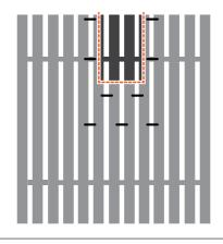
**(Option B)** If the cut you are making is on the edge of the tile, step 2 (Option A) can be ignored. Simply make your measurements on the back of the tile (in reverse) and proceed to step 3.
