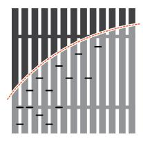
Before cutting, secure the back of the tile with crown staples and stagger them.
