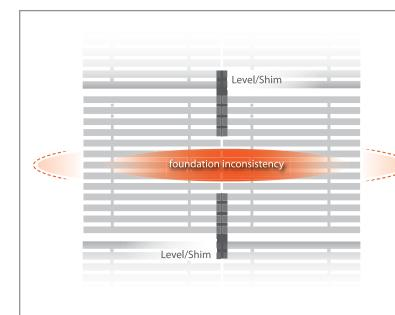
Use your levelling strips to compensate for uneven surfaces, bumps, obstructions. As if the tile were a teater-totter mounted on a fixed point (the bump) use these strips on either end if not both to stop the rocking motion. Levelling material may also be overlapped and shared between two tiles when the direction is consistent as in this case. Furthermore, stacking the material will give you the ability conform to any irregularity the tile(s) are positioned on top of.
