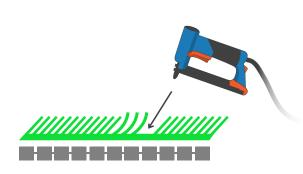
Drive your staples diagonally (underneath the blades) to secure.
