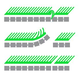
Tip: You'll notice that at one edge of the tile, its blades of grass may get trapped underneath the next as it's butted up together. By gently lifting this tile and freeing the material, the nap will overlap the tile you have just placed down and create a uniform look.
