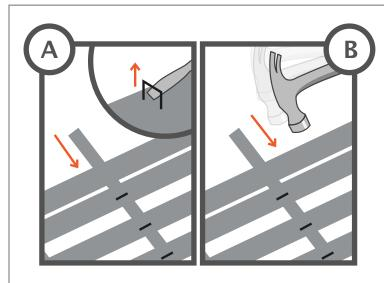
Tip: (A) For further flexibility with fitting a tile, the small staples holding the slats to the PVC tubing on the back can be raised using a flat head screwdriver. By lifting them up, you can slide the slat(s) on the tube in the desired direction.
