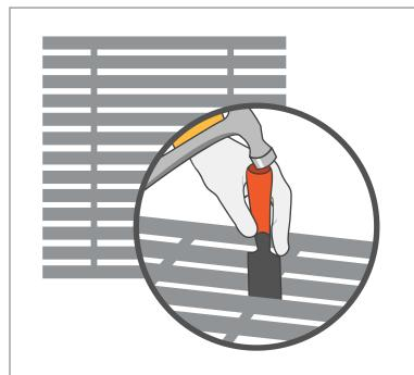
Note: If a tile falls in a horizontal relationship to the boundary and requires resizing, you may split the PVC tubing of the underpart (wood tile) with a chisel of knife to allow for an accurate fitting.
